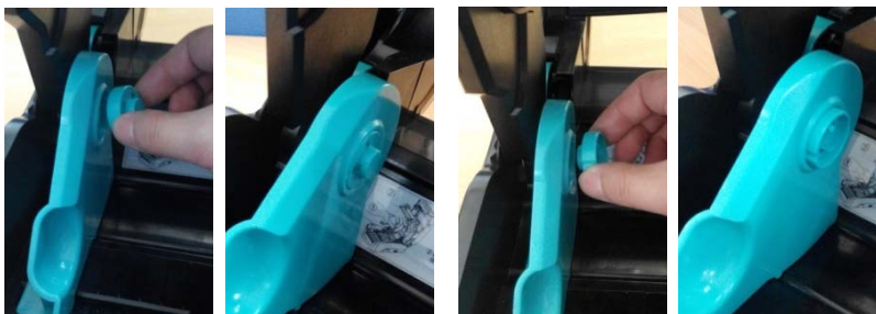
Install 12.7mm paper roll core
